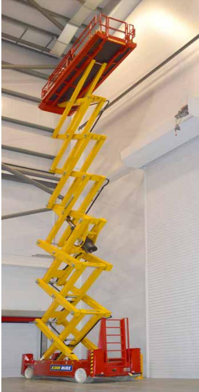
These impressive Scissor Lifts provide a maximum working height of 19m or 22.5m (depending on the model) while still only 1.22m wide. An automatic levelling system provides the user with additional stability allowing indoor or outdoor use. Ideal for high level narrow warehouse aisle applications or inner-city applications on narrow pathways etc.
