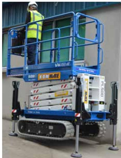
This Tracked Scissor Lift has auto levelling outriggers which extend to 400mm allowing levelling on the most uneven surfaces. Retractable outriggers allow travel through narrow entrances only 800mm wide making this machine ultra versatile.
