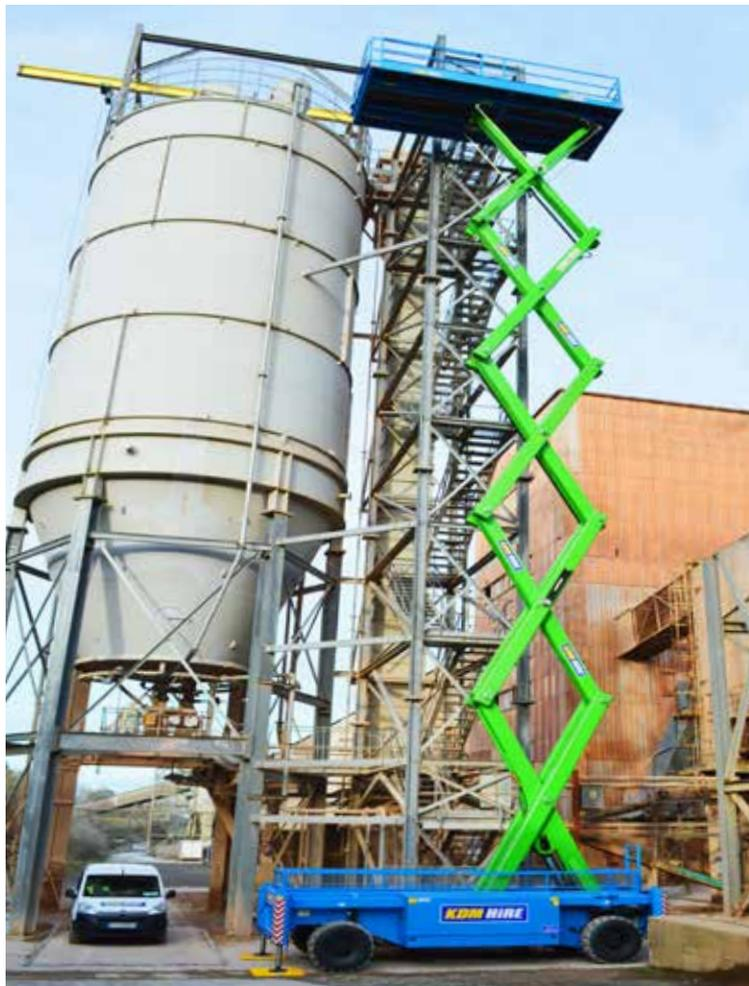
This mega HL-275 D25 Diesel Scissor Lift offers a working height of 27.5m, a working area of up to 8.25m x 2.35m (extended) and a safe working capacity of 1000kg.
