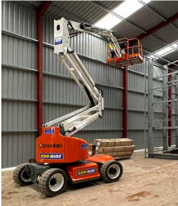
With working heights of up to 15.9m, these quiet, emission-free lifts can provide outreach capacity of up to 6.1m and full 360° articulation. Perfect for internal jobs, which require high reach and perfect positioning.
