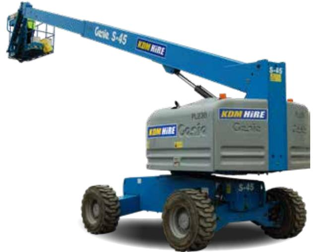
With 4WD and flick-out jibs as standard, these Rugged Telescopic Booms are ideal for a host of applications, including structural steel and general maintenance work.
