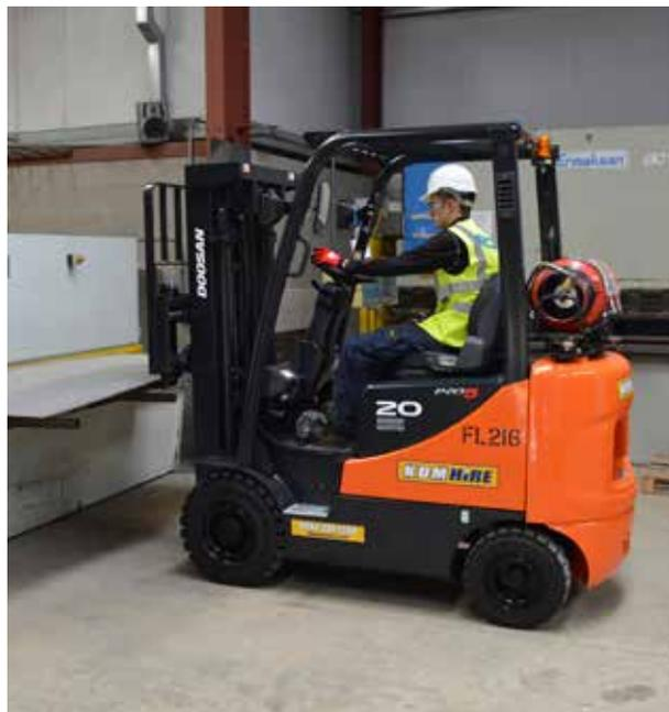
Producing less emissions than conventional diesel forklifts, these Gas Trucks are ideal for use in ventilated warehouses or factories where personnel are working.
