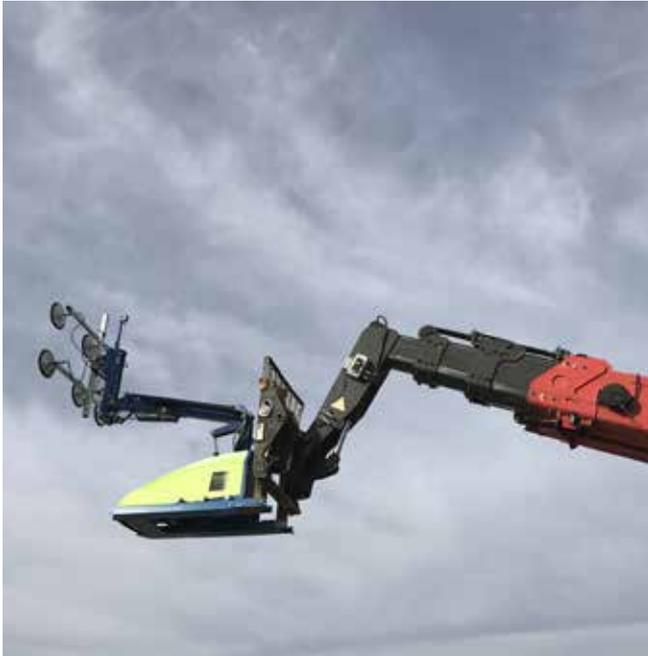
This glass positioner fits directly to the forks of a telehandler or forklift for installation of glass at height or where ground conditions are difficult. With a 350kg capacity and operated by a cabled remote control, the unit allows safe handling and manipulating of glass in places a standard unit cannot reach.
