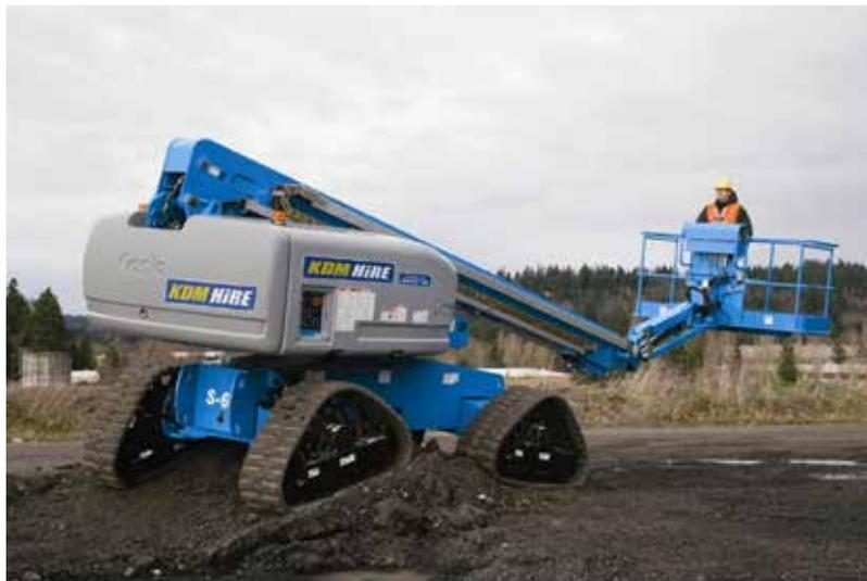
When you need the ultimate in rough terrain ability, the 4-track telescopic boom lift is the only answer. With unique 4-point tracking and oscillating axle this machine offers superior traction allowing it to go where other booms will not. Suitable for the most arduous sites and field conditions, ideal for transmission line work.
