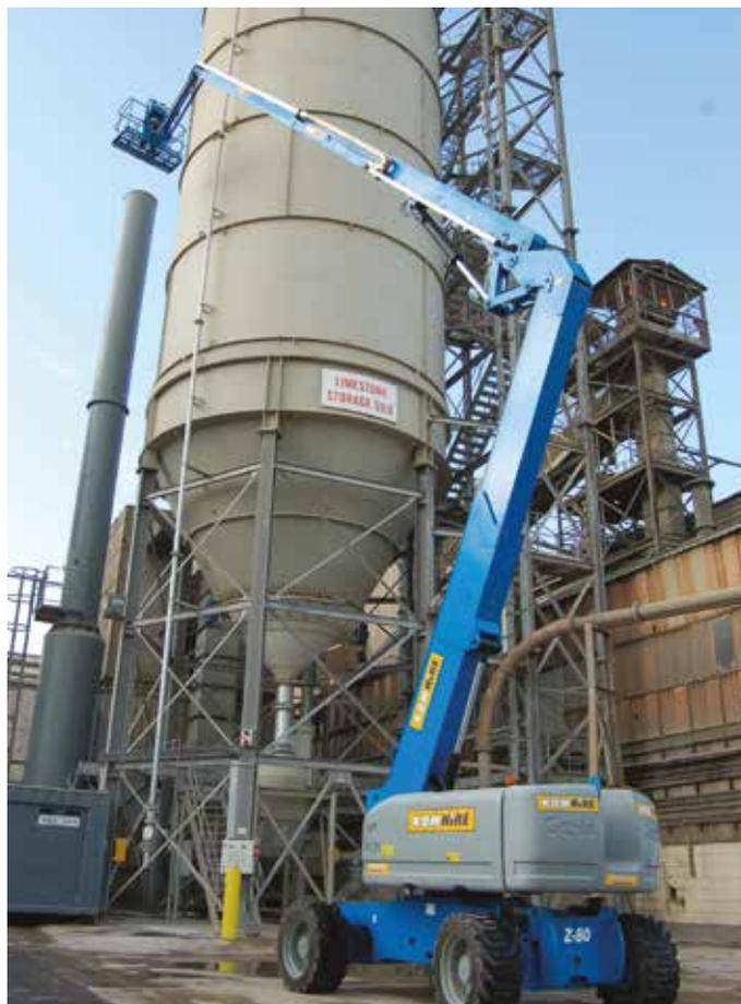
With an impressive outreach of 18.3m or 60ft, this large Artic Boom provides unsurpassed up & over positioning. This machine is ideal for maintenance or repair tasks on old buildings or industrial applications.
