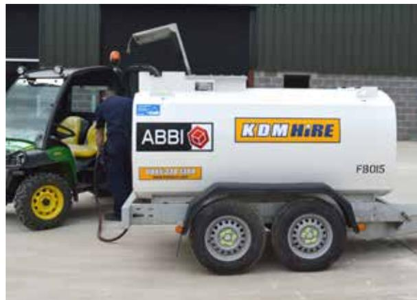
When transporting bulk fuel to site, these Tandem Axle Fuel Bowsers allow you to do so in a safe, legal manner. This Fuel Bowser is fully bunded and compliant with all road towing regulations. Can be used for refuelling or connection to static equipment.
