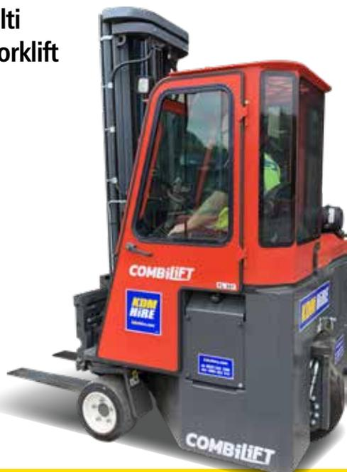
This innovative compact forklift provides the versatility to operate as a narrow aisle forklift, handle long lengths such as steel beams and timber plus still offering the manoeuvrability of a conventional forklift. The low profile and compact design also improves safety and increases productivity. Suitable for indoor and outdoor applications the compact multi directional forklift has the ability to handle a diverse range of goods in most industries.
