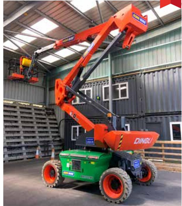
This all electric Boom allows emission free and quiet operation for heights up to 20m. It also boasts the reach characteristics of standard machines but with the advantages of non-marking tyres and continuous 360° rotation while being very economical to run.
