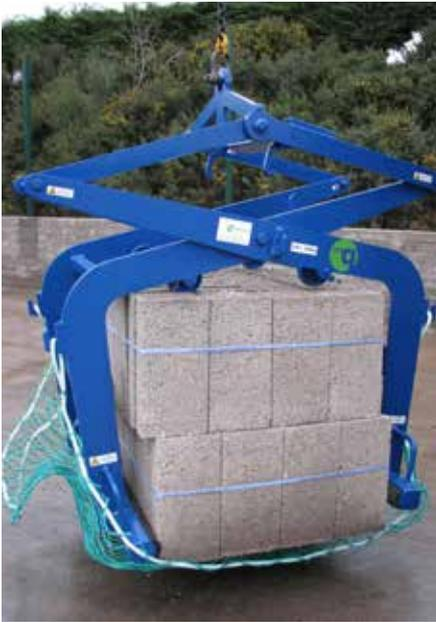
Single or double scissor Block Grabs are the solution for positioning bales of blocks and other concrete products on site. Used with an excavator, handler or other lifting machine.
