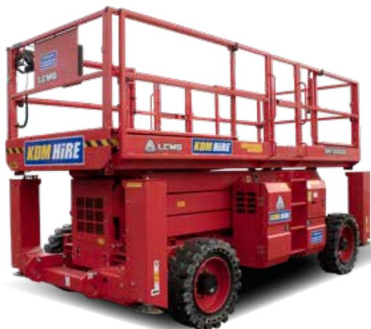
With twin roll-out deck extensions providing a platform size up to 7.38m long and lift capacity of up to 1.1t, these Scissor Lifts will handle the toughest jobs.
