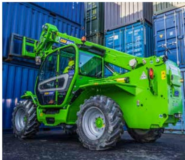
These Heavy Lift Telehandlers are the ultimate site workhorse providing up to 7200kg lifting capacity - 4000kg at full height (9.55m). Ideally suited for safely handling larger heavy loads or large volume shovelling applications.
