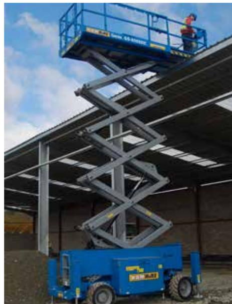
Available in electric hybrid options, these machines provides excellent rough terrain capability whilst offering zero emissions and quiet operation for noise sensitive environments. Other features include a maximum working height of 14.2m and a 4.31m extended deck size.
