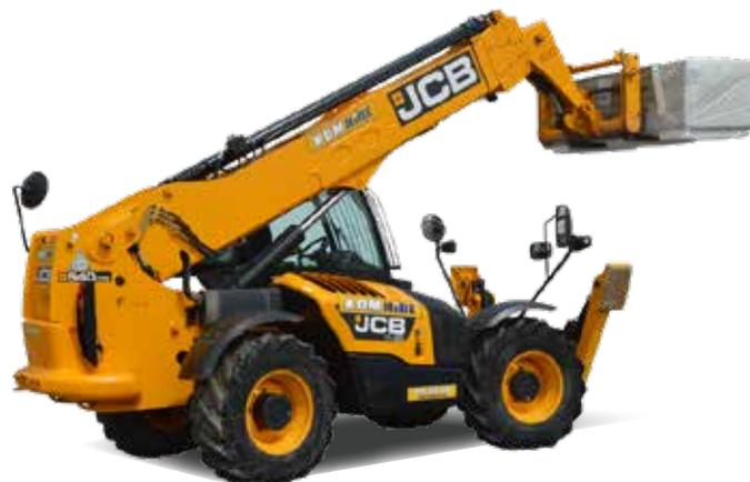
With lift capacities up to 4t and forward reach of up to 13.08m, these 17 & 18m handlers are the ultimate performers around the site. These well balanced machines ensure precision placement of loads. Side shift and frame levelling are available on most models.
