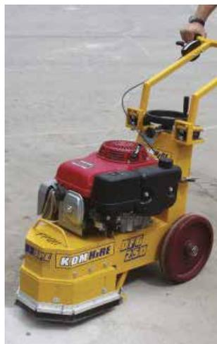
For preparation, debris removal and smoothing of concrete floors, these Grinders can be used with diamond heads or carbide stones.
