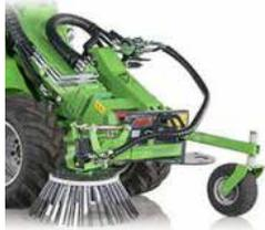
The weed brush is an efficient tool for removal of weeds or moss from paved areas, yards or tarmac driveways. Three positions make it ideal for cleaning along edges, kerbs or fences.
