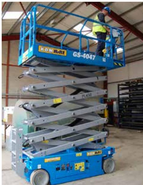
At only 1.19m wide and offering a working height of nearly 14m, this Scissor Lift is ideal for high-level maintenance or fit-out of warehouses or factories. A lifting capacity of up to 350kg and a 91cm slide out deck extension make this machine exceptionally versatile. Standard features include solid non marking tyres and folding handrails.
