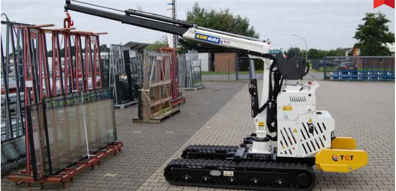
The unique tracked pick and carry crane allows safe positioning and handling of goods or materials on soft ground or rough terrain. The tracked crawler chassis provides low ground pressures while retractable tracks allow access to narrow driveways or paths. With a lift capacity of 900kg, forward reach of over 3m and lift height of 4.3m, the tracked pick and carry crane is ideal for positioning glass, marble slabs or structural beams in otherwise hard to reach places.
