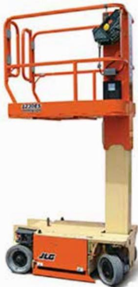
Hydraulically operated vertical mast provides an exceptionally smooth operation while clean and quiet for a variety of environments. Front wheel drive provides outstanding manoeuvrability and long cycle duties.
