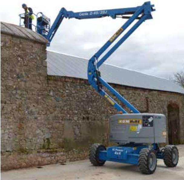
The 45ft Boom is the workhorse of the access industry. 4WD, puncture-proof tyres, zero tail swing and flick-out jibs are just some of the features making this machine perfect for the toughest sites.
