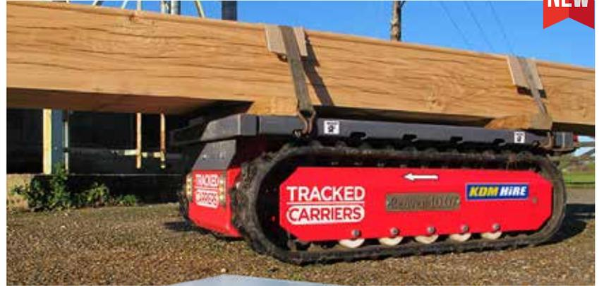
This state of the art tracked mover removes the need for manual handling, reduces labour costs and increases productivity when handling or transporting larger components into tighter spaces. Battery powered with radio remote control, the tracked carrier will handle difficult sites and gradients with ease while keeping the operator a safe distance away. Swivel platform and dolly accessory options are available to make long load handling safe and simple.
