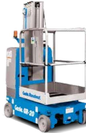
Driveable when fully elevated at working heights of up to 8.07m, these machines offer increased productivity for fit-out, maintenance or stock picking tasks.
