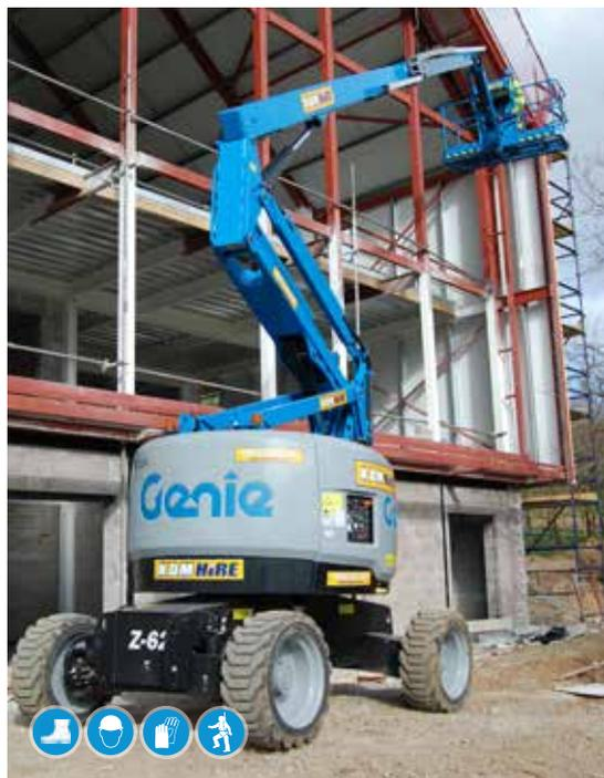
For up & over positioning where additional outreach is required, these large Articulating Booms have zero-tail swing allowing rotation in restricted areas where other similar machines cannot go.
