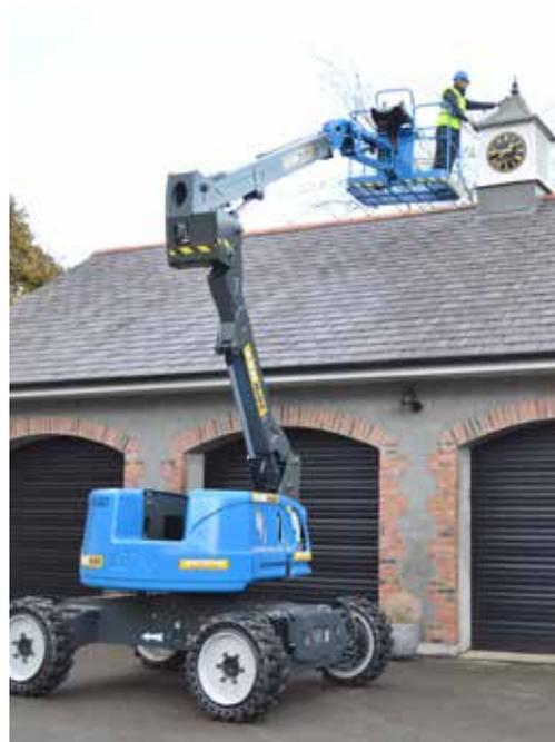
These Booms offer 4WD capability for applications up to 12.6m. With zero tail & nose swing and at only 1.99m wide, these Diesel Booms are ideal for working in confined areas.
