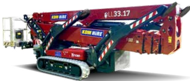
Battery Hybrid power allows for indoor operation
