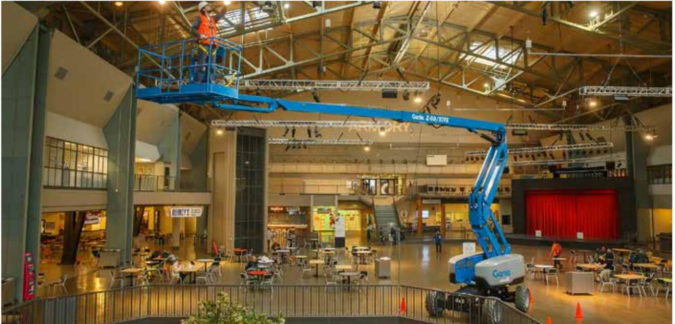
This Hybrid Boom is ideal for outdoor and indoor applications such as construction sites, sports arenas, malls, manufacturing facilities and even challenging pedestrian areas with the demand for low noise and clean performance.
