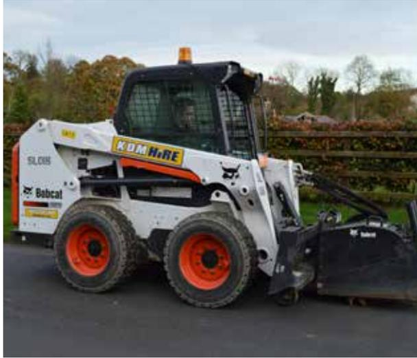
These High Flow machines offer greater power and stability for use with road planers and other hydraulic attachments. Advanced hand controls, full cabs and heavy duty tyres are other standard features of these Skid Steers.
