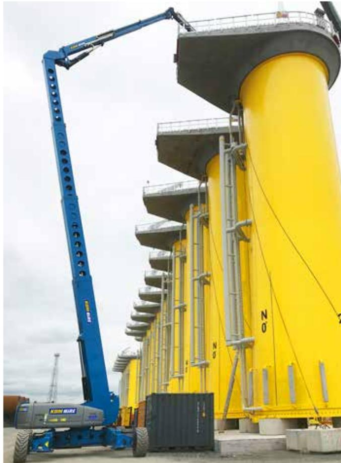
The Z135/70 gives an impressive working height of 43.15m and a massive up and over reach of 18m at 23m high or 21.26m of reach at nearly 10m vertically. The 20m extending jib provides effortless positioning while the chassis extends in a unique X pattern for ease of set up.
