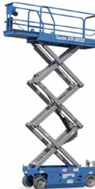
With working heights up to 10m and only 810mm wide, these Narrow Scissors are perfect for manoeuvring into awkward areas. Non-marking tyres allow travel over sensitive floors.
