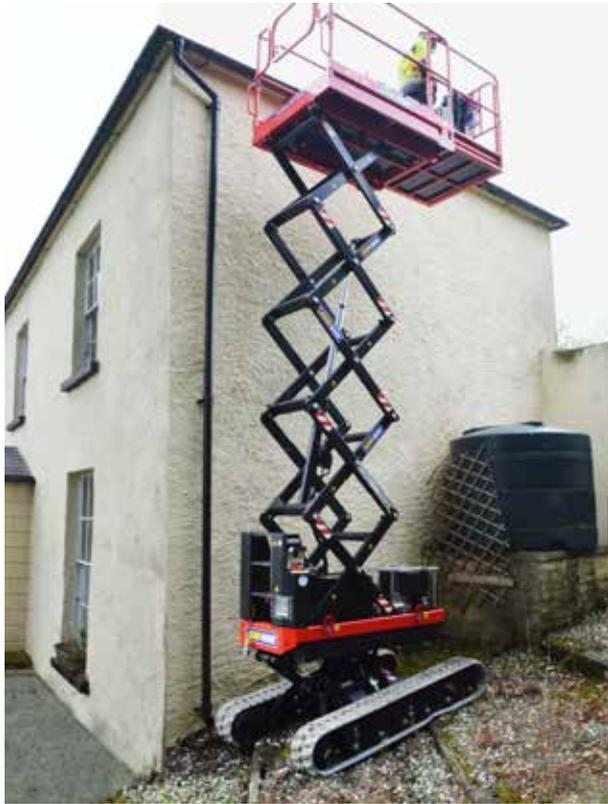
This unique Bi-level Tracked Scissor provides safe access solutions on slopes of up to 20°. Capable of levelling both longitudinally and laterally, this machine will operate in the roughest and most uneven conditions. The crawler traction allows access to areas not suitable for traditional 4 x 4 machines.
