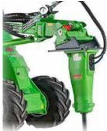
The hydraulic breaker is an effective tool for demolition or refurbishment applications. Ideal for concrete, Tarmac or masonry walls.
