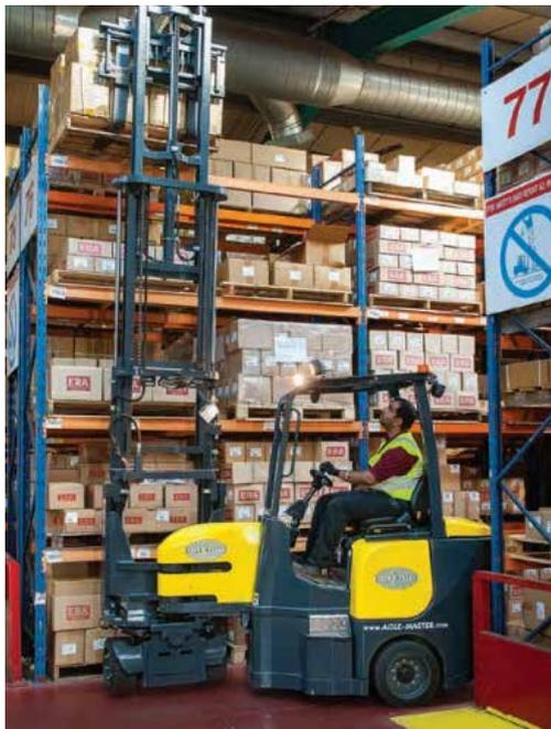
With the ability to operate in very narrow aisles (as narrow as 1.6m) this articulating forklift maximises storage space and eliminates time consuming double handling of materials. Capable of working indoors or out this electric truck is the ideal solution for large warehouse racking operations.
