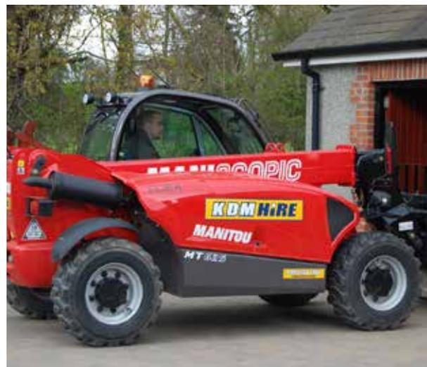
As your work conditions become increasingly demanding, this highly manoeuvrable compact machine is ideal for your site where space is at a premium, providing a loading capacity of 2500kg and a maximum lift height of 5.85m. The cab has been designed to offer excellent all round visibility and driver comfort plus easy access is provided by the low level door.
