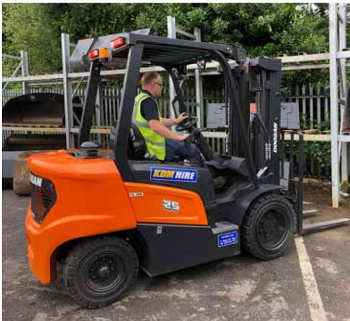
These efficient Diesel Forklifts offer the most reliable option when shifting goods and materials around industrial yards or factory units. Most trucks are fitted with side shift for extra productivity and puncture proof tyres for reduced down time. Numerous mast configurations and cab options are available.
