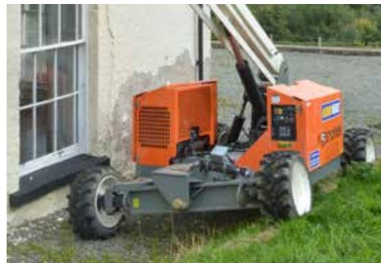
The unique SL30SL Speed Level offers automatic powered platform levelling without the need for outriggers. Level up to 13° from side-to-side and up to 9° from front-to-back swiftly for a stable working platform. Driveable at full height (11m), the Speed Level offers a spacious platform (1.72m x 4.32m) and a powerful 4-wheel-drive ideal for cladding and glazing applications on rough terrain sites even on compound slopes.
